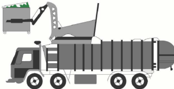
Front-lift-loading waste collection vehicle
